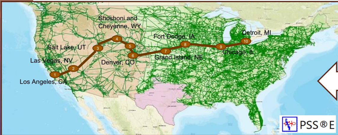
Scenario: 10-terminal radial MTdc scenario planned with point of interconnection in the ac grid
